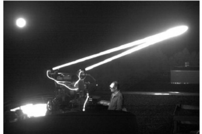
Fig. 11. Optical Ground Station Oberpfaffenhofen (OGS-OP) during the Kiodo 2009 trials. Visible on the infrared picture is the beacon laser's backscatter due to haze.
