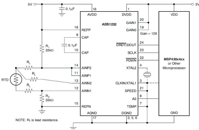
Fig. 4 RTD Three-Wire Schematic from Atmel Datasheet [6]
