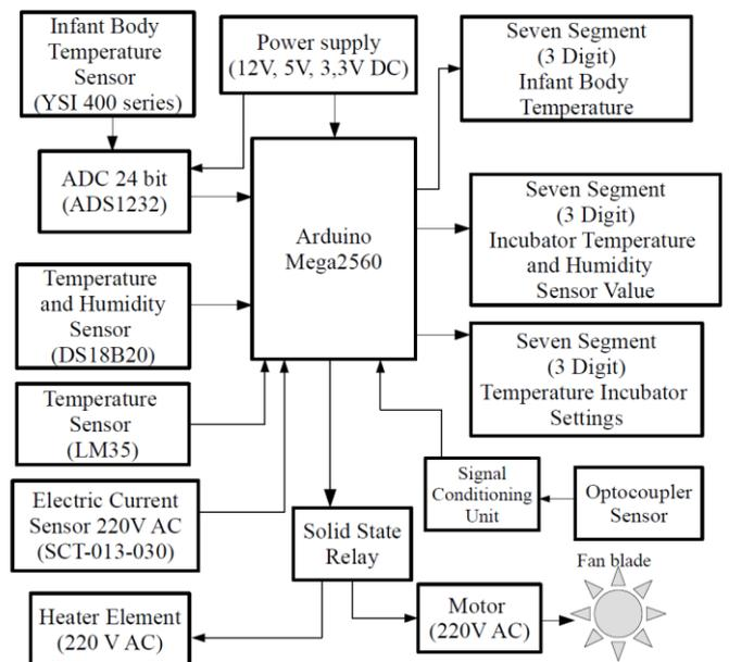
Fig. 2 Block Diagram of Infant Incubator Temperature Controlled and Body Temperature Monitor
