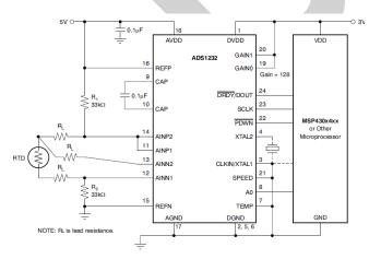
Fig. 4 RTD Three-Wire Schematic from Atmel Datasheet [6]
