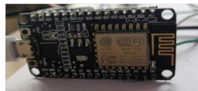
Figure.2 ESP8266 NODE MCU
